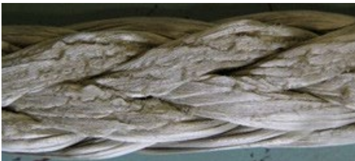
Fig. 14: Example of heat damage - melted fibres
