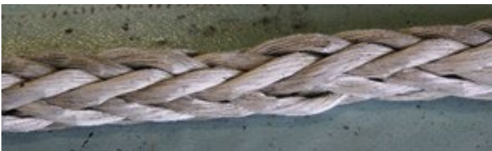
Fig. 13: Example of non-uniform deformation
