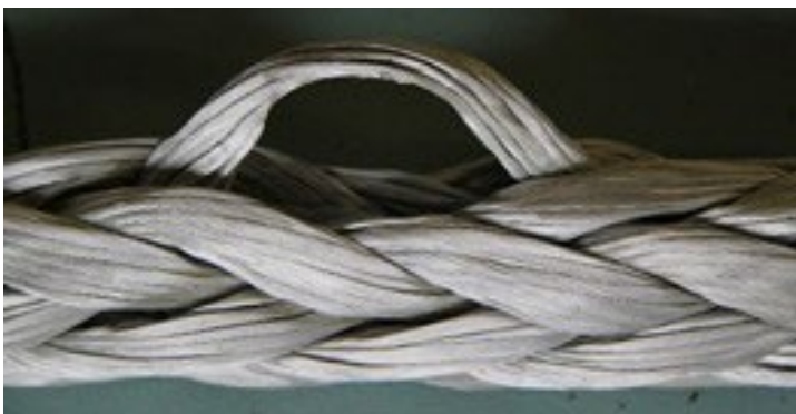
Fig. 12: Example of pulled yarns/strands
