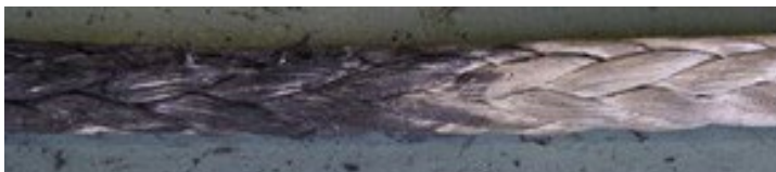
Fig. 16: Example of damage due to chemical influence
