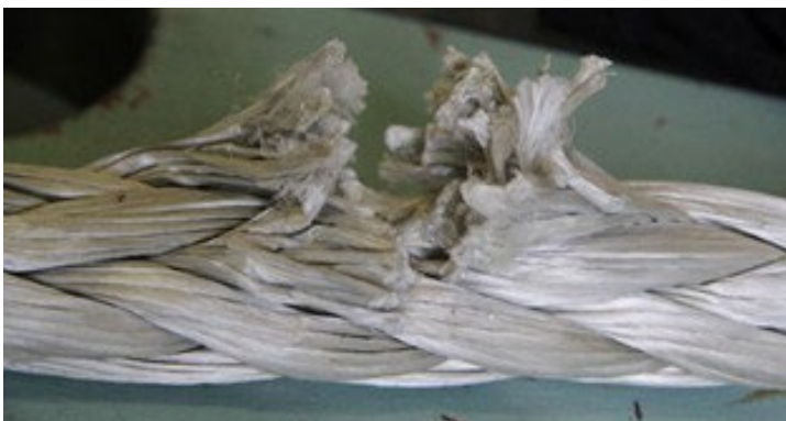
Fig. 10: Example of cut strands
