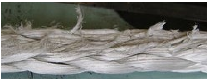
Fig. 9: Example of severe damage due to external wear and tear
