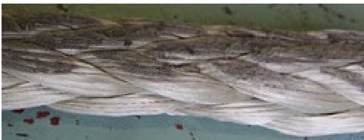
Fig. 8: Example of slight damage due to external wear and tear
