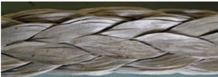
Fig. 15: Example of heat damage - glazed fibres
